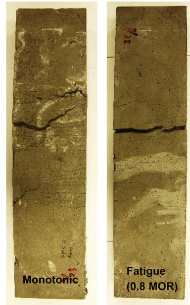
**Fig. 9.** Crack pattern at failure for lightweight ECC under flexural monotonic bending and fatigue loading at 80% of flexural strength.
